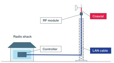
By adopting PoE technology, the connection is made with a single cable, providing a more flexible mounting solution for the RF module. Additionally, the PoE technology makes it possible to use a higher voltage, reducing the current needed for a stable power source for the RF module.
